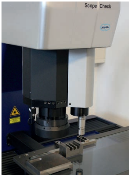
Figure 3. For tactile measurements, the components must be properly clamped to prevent them from moving. The fixtures are later used for process control in production as well.
