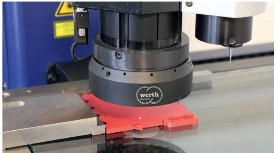
Figure 2. Measuring the flatness of plastic sheets. The laser on the 3D multisensor coordinate measuring machine reduces the inspection time by about two-thirds.
