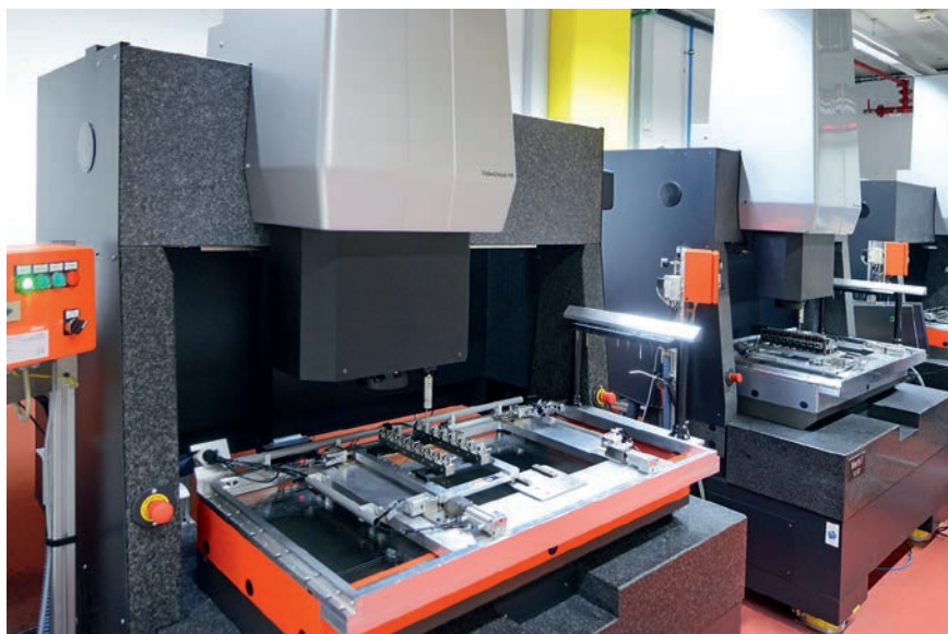
Figure 2. For high-precision measurement tasks: the highest-precision class of VideoCheck machines can reach a maximum permissible error in the range of tenths of microns. (© Blum)
