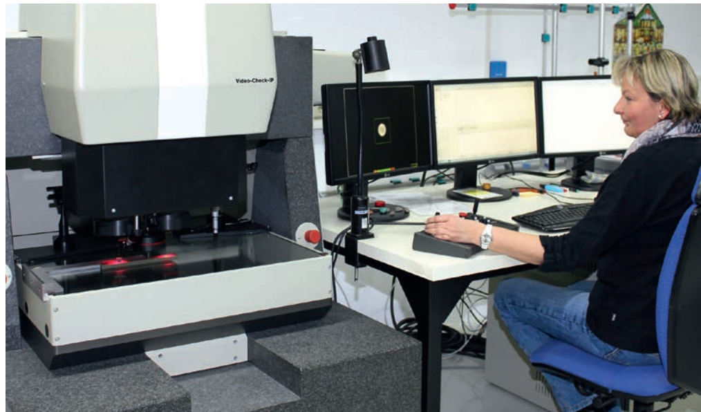
Fig. 1. The fixed portal measuring machine is equipped with telecentric optics as well as a fiber probe and a conventional trigger probe.
