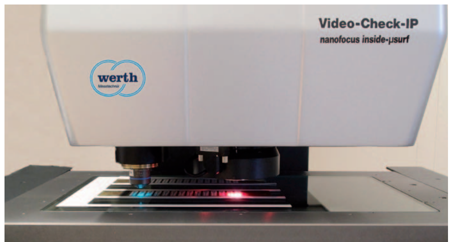
Figure 1. VideoCheck® IP: The two sensors of the Werth VideoCheck® IP 400 can be seen in the photo. On the right is the image processing sensor (red light) and on the left is the Nanofocus measurement head (blue) in sequential operation. (Photos: Roche)
