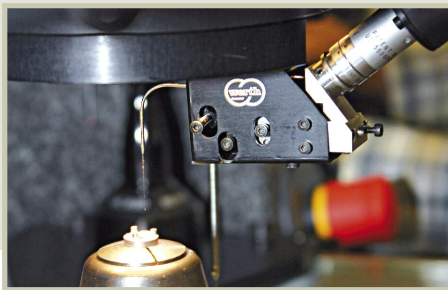
Image 2. The »WFP« fiber probe is a microprobe for high-precision applications. It makes it possible to perform contacting measurements of extremely small geometries, with very small contact forces, at high precision
