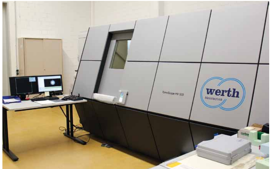
▲ The computed tomography system is used for geometric measurement tasks and material analysis.
