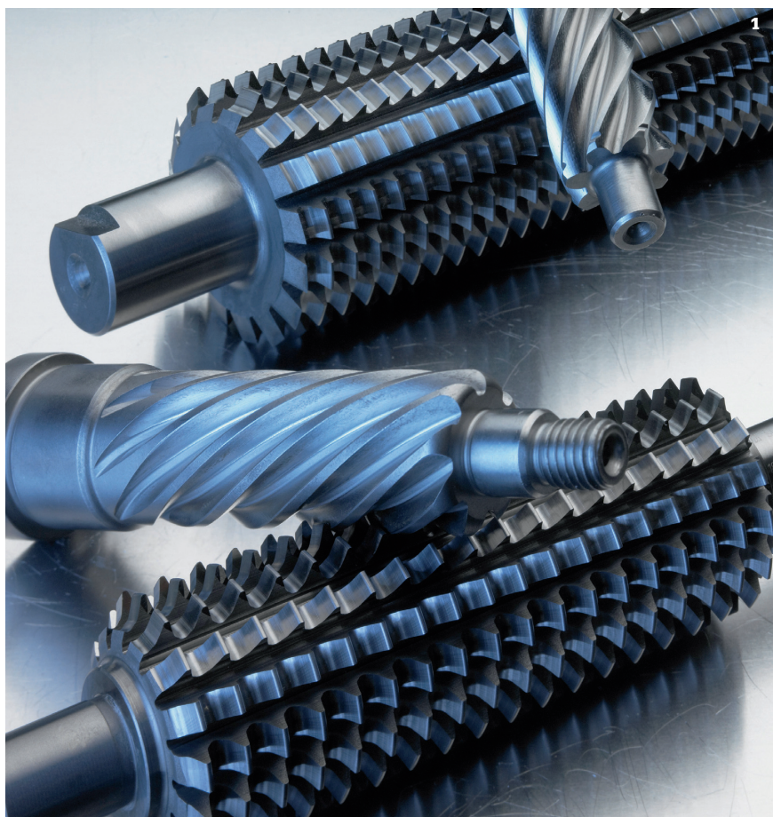
1 Schnyder SA specializes in customer specific gear cutting tools. 2 This vertical VideoCheck V HA from Werth is in the metrology room at Schnyder.
