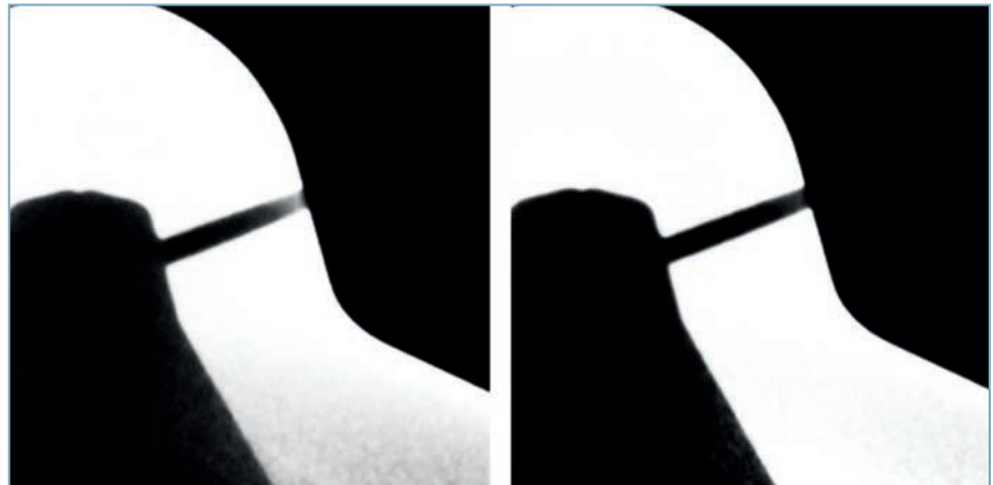
Figure 3. Volume cross section through an injector nozzle prior to (left) and after (right) Empirical Artifact Correction EAC
