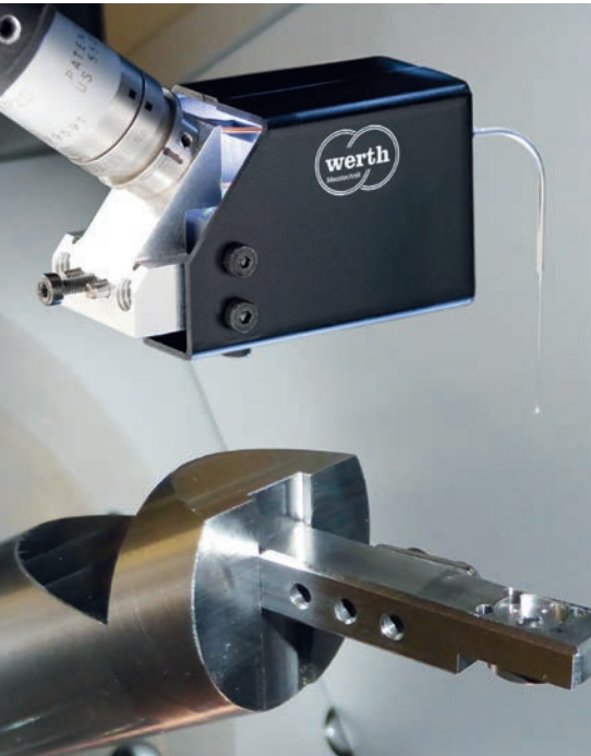
Figure 3. Gasoline fuel injector mounted on a rotary/tilt axis on the multisensor coordinate measuring machine
