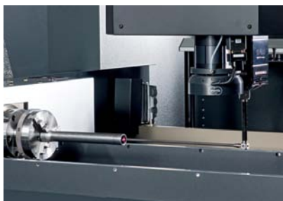
Measurement of internal teeth using VideoCheck + SP 80
