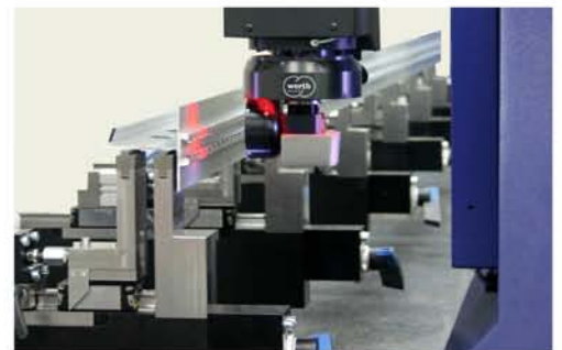
Clamping the profile takes only a few minutes
