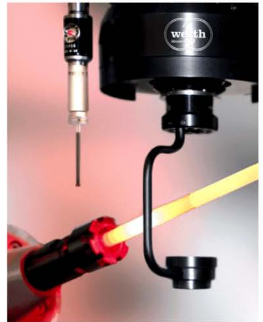
In order to measure the fine structures of stents, they are drawn onto special mandrels. Image: Werth Messtechnik GmbH
