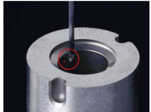
Hole measurement using the WIP Werth Interferometer Probe
