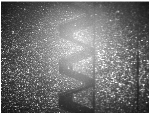
Interfering reflection when measured with brightfield incident light
