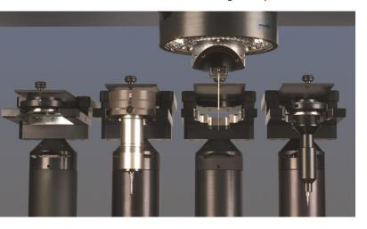
WFP/S Werth Fiber Probe on the WMS magnetic interface, with other sensors in the background
