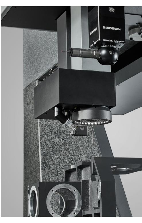
Dual ram with tactile, optical and tactile-optical sensors
