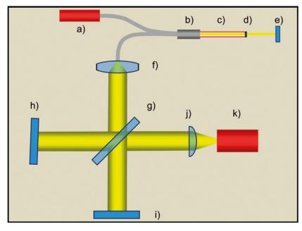
Principle of the interferometer point sensor (WIP): a) superluminescent diode, b) fiber coupler, c) probe, d) probe exit and reference surface, e) workpiece surface, f) collimator lens, g) beam splitter, h) mirror 1, tilted, i) mirror 2, j) cylinder lens, k) line camera
