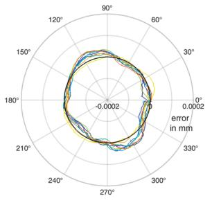
Roundness measurements with minimal measurement errors of about 100 nm
