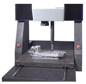
With the new transmitted light concept, heavy workpieces can be measured directly on the measuring table.
