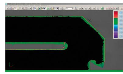
A raster image superimposed on a DXF file, with colorcoded deviation plot from contour comparison
