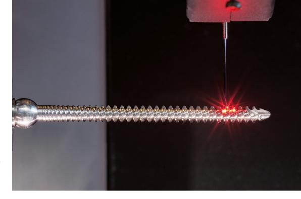
Measuring with the Werth Fiber Probe® (WFP) a thread on a pedicle screw for stabilizing vertebral bodies
