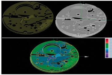
Figure 6: Optical distance sensors provide a 3D point cloud of the workpiece surface (top left), which enables a target-to-actual comparison with the CAD model (top right) in addition to dimensional measurements, along with a color-coded deviation plot (bottom).
