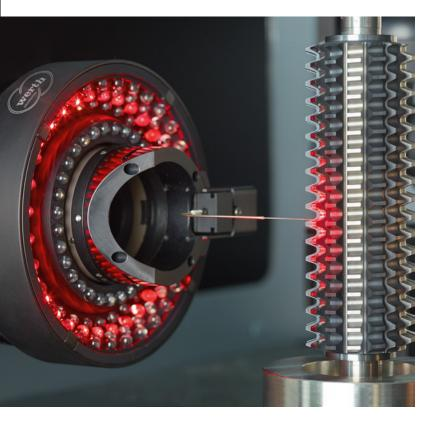
Figure 5: The Werth Fiber Probe<sup>®</sup>, or WFP (patented), with a probe sphere as small as  $20 \ \mu m$  in diameter, is the most accurate micro-stylus on the market.
