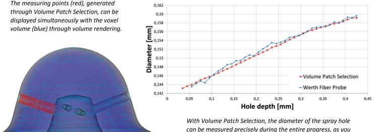
can be measured precisely during the entire progress, as you can see from the comparison to the Werth Fiber Probe<sup>®</sup>.
