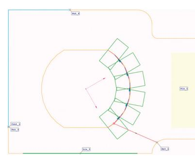
With 2D-CAD-Online<sup>®</sup>, various geometrical features can be measured directly by clicking the Werth 3D graphic.
