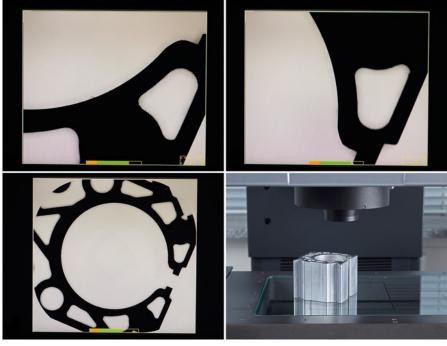
Figure 4: The patented Werth Laser Probe is integrated in the beam path of the Werth Zoom image processing sensor.
