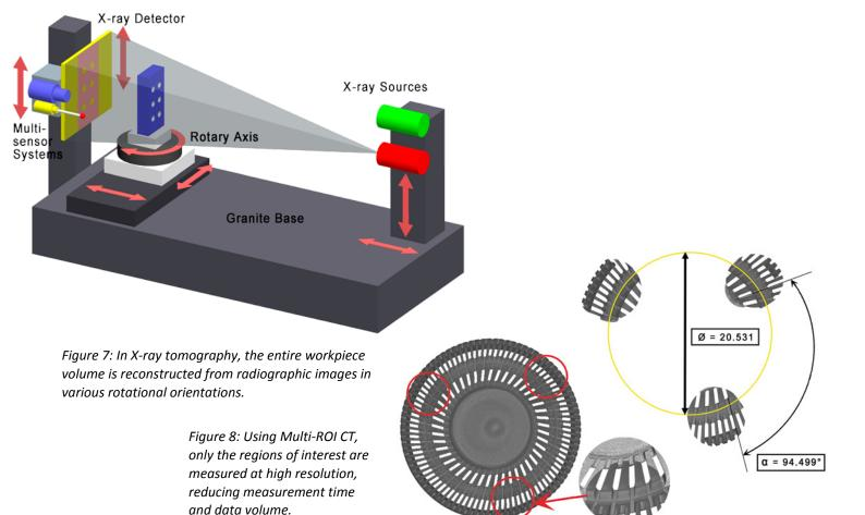
200 in 2005, the first machine with X-ray tomography developed especially for coordinate metrology, with optional multisensor systems [9]. This machine already had specifications and measurement uncertainties comparable to conventional coordinate metrology. "Measure completely and accurately" was the new motto, as now for the first time all of the areas of the workpiece that were difficult to access, including internal geometries, were able to be captured (Figure 7).
