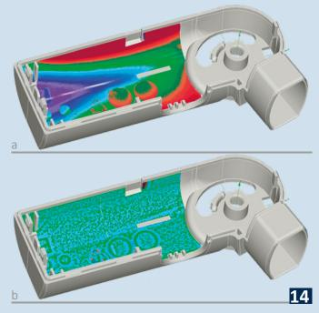
Using WinWerth® FormCorrect with its high precision, the deviations of the plastic injection molding workpiece (a) are often corrected in only one iteration (b).
