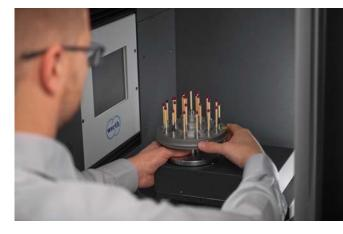
William Hemelik with the TomoScope® XS Plus (above) Placing a multi-sphere calibration standard on the rotary table (down)
