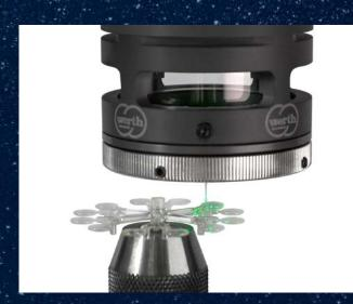
With the WFP<sup>®</sup> 3D, all parameters of the plastic lenses, including the entire surface geometry, can be measured in a single measuring sequence with manufacturing tolerances down to the sub-micron range. Mainly, the complex forms of the aspherical surfaces and their concentricity are measured. As with the LED lenses, the mounting position of plastic assemblies can also be captured using CT. Thus, the distances between the lenses, gap dimensions, and coaxiality can be measured.
