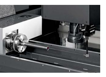
Measurements of inner contour and pitch deviations with conventional rotary axis and wobble correction by WinWerth®
