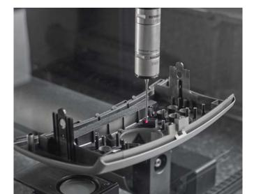
Fast alignment of the workpiece and 3D-contour measurement using the image processing system and the patented Werth Zoom with integrated Werth Laser Probe (above).
