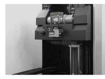
High resolution microfocus X-ray tube (down) and high power macrofocus X-ray tube (above)
