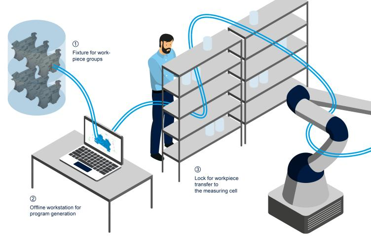
Small measurement objects (such as plastic injection molded parts) can be measured simultaneously in multi-object measurements of, for example 8, 16, 32, or 64 workpieces. This feature further reduces cycle times to a few seconds per workpiece. For such measurements, the Werth transmission tubes provide very good structure resolution even at relatively high power. This allows for defects such as burrs to be reliably detected while retaining fast measuring speeds.
