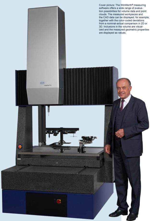
The ScopeCheck® FB DZ machine series was expanded. The multi-ram concept is now available for large workpieces. This allows multisensor measurements to be carried out without restriction and avoids collisions.
