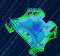
Modern Coordinate measuring machines with computed tomography sensor technology provide a complete digital twin of the workpiece in a short time. This is suitable both for dimensional measurements and for nominalactual comparisons with color-coded deviation display. Picture: Weidmüller News about the Werth Group
