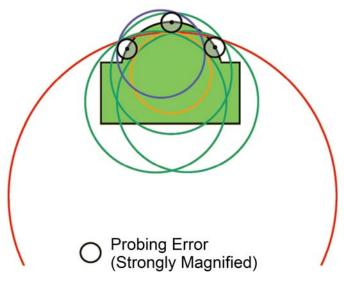
When measuring radii use the greatest possible arc to reduce measuring uncertainty
