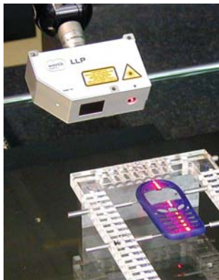
Figure 2. Using the laser line sensor, free-form surfaces can be captured quickly, without contact.
